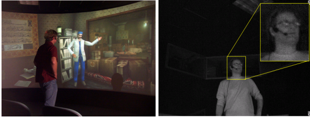
Fig. 8. left Theater environment for head tracking application. Subject is in nearly complete darkness except for the illumination from the screen. Image courtesy of USC’s Institute for Creative Technologies. right Images from high resolution IR camera placed below the screen.
