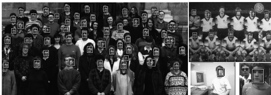
Fig. 7. Sample results of the face detector based on integral projections. The images were taken from the CMU/MIT face database [13]. More results available at [14].
